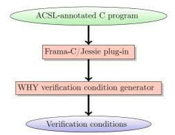
Fig. 1 Chain of tools: from the C program to the proof obligations
