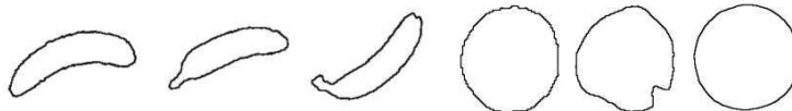
Fig. 5. A selection of the multiple exemplars used to represent the model for bananas and oranges. Multiple shape exemplars are required to handle intra-class shape variability.
