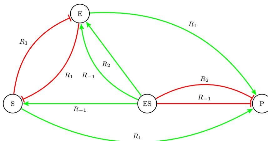
**Fig. 6** Influence graph of Fig. 4 but with arcs ending in  $ES$  and  $P$  substituted. Resulting self loops are, as usual, not shown, but note that the two negative arcs from  $ES$  to  $P$  correspond to two negative self loops in the original graph. The only positive cycle contains twice  $R_1$ .
