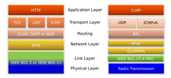
Figure 1: Comparison of the traditional TCP/IP stack used by most Internet hosts and the corresponding protocols for IoT networks.
