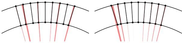
**Fig. 6** Visualization of the relationship between  $\phi_j$  (inner points) and  $\phi = \hat{\eta}\theta_j$  (outer points) for the left and right cameras. The angular errors (represented by the translucent sectors) are greatly reduced with respect to those in Fig. 4 (note that the inner points, representing  $\phi_j$ , are unchanged).
