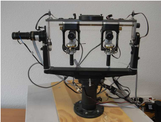
Fig. 1 The POPEYE active binocular robotic head (designed and built in the Institute for Systems & Robotics, University of Coimbra, Portugal). The binocular vergence is controlled by a pair of motors, one below each camera. The pan and tilt angles of the head are controlled by another pair of motors.
