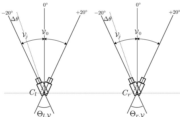
**Fig. 3** An illustration of the motor-camera calibration procedure. For each camera, a set of images are extracted which are representative of the viewable area. The relationship between the motor-angle  $\theta$  and the homography-angle  $\phi$  is modelled by the method described in section 2.3.
