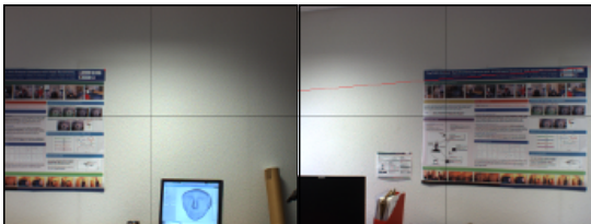
(b) The left and right cameras are rotated by -10 and +12 degrees respectively, and the homographies representative of these rotations are calculated.
