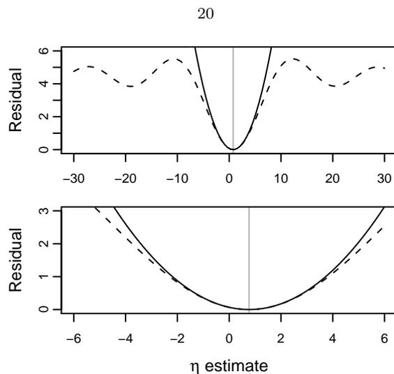
**Fig. 5** Comparison of the angular (dashed) and Euclidean (solid) metrics (9), on the actual data-set. The upper plot shows periodic form of the angular error. The global minimum is well-approximated by a parabola, as in (10). The least-squares estimate (12) is the minimum of the parabola, indicated by the vertical line. For the present data, the difference between the two metrics is insignificant. The lower plot shows a magnified view.
