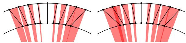
**Fig. 4** Visualization of the relationship between  $\phi_j$  (inner points) and  $\theta_j$  (outer points) for the left and right cameras. The connecting lines would be purely radial if all  $\{\theta_j, \phi_j\}$  pairs were equal. The area of each translucent sector is proportional to the corresponding angular discrepancy  $|\phi_j - \theta_j|$ .
