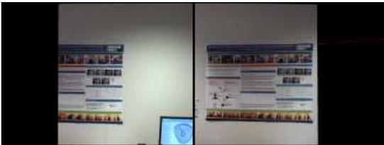
(c) The estimated homographies are then used to un-rotate the current images to the original fronto-parallel views (note: the field of view is truncated).
