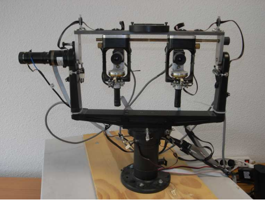
Fig. 1 The POPEYE active binocular robotic head (designed and built in the Institute for Systems & Robotics, University of Coimbra, Portugal). The binocular vergence is controlled by a pair of motors, one below each camera. The pan and tilt angles of the head are controlled by another pair of motors.
