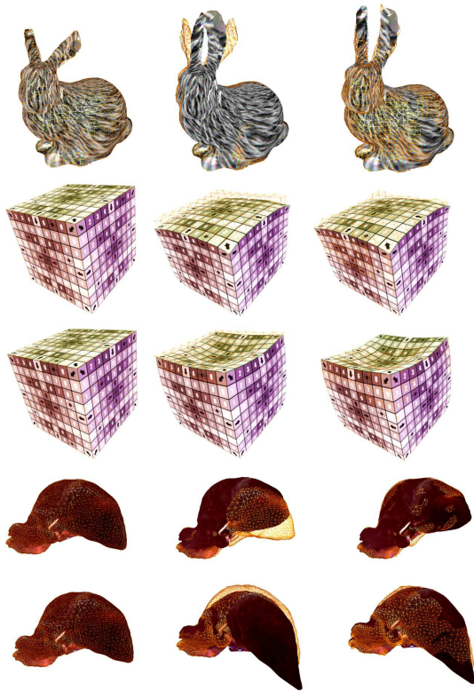
Figure 7: Synthetic datasets on various meshes and deformations. The left image represents the initial condition, the middle one an intermediate motion and the rightmost one the final configuration. The reference mesh is displayed with plain faces whereas our algorithm provides deform meshes displayed in wireframe (orange lines). The results exhibit a good matching of the reference mesh and the tracked one.
