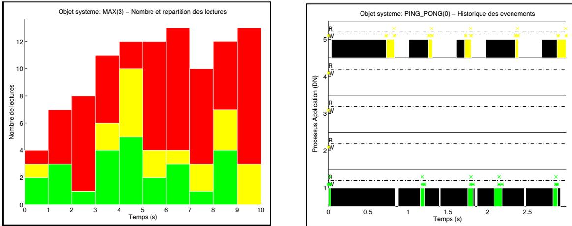
Figure 7: Number and origin of the read accesses performed on an object vs execution time (in : here a ping-pong effect between two processes) Figure 8: Object activity vs execution time (black : inter-group accesses)
