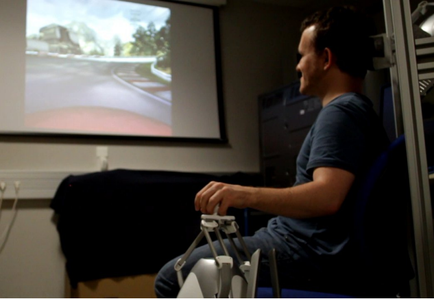
Figure 4: The user, comfortably installed on our device, is experiencing passive navigation enhanced by a haptic effect of motion.
