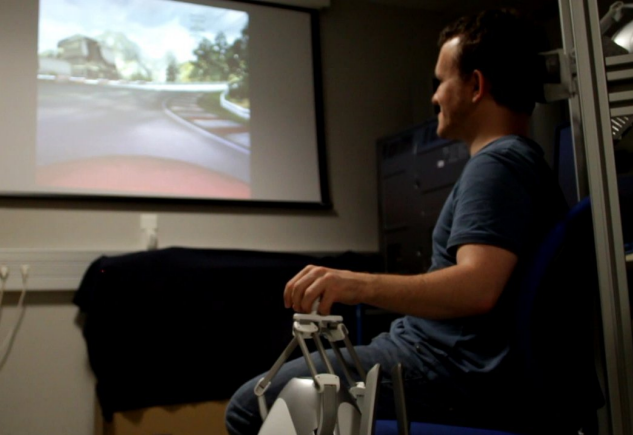
Figure 4: The user, comfortably installed on our device, is experiencing passive navigation enhanced by a haptic effect of motion.
