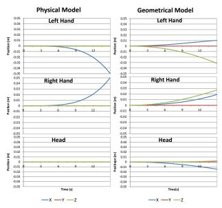
Figure 3: Output of the models (*Physical* on the left, *Geometrical* on the right) for a left rotation around Y-axis of 15 seconds. The position in meters is plotted for each actuator LA, RA and H, and for each axis.
