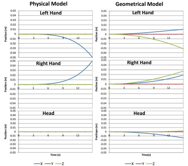
**Figure 3: Output of the models (*Physical* on the left, *Geometrical* on the right) for a left rotation around Y-axis of 15 seconds. The position in meters is plotted for each actuator  $LA$ ,  $RA$  and  $H$ , and for each axis.**
