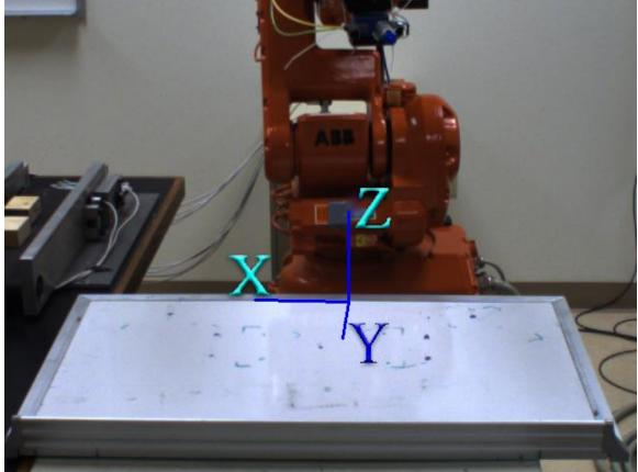
Figure 4: Robot Coordinate System
