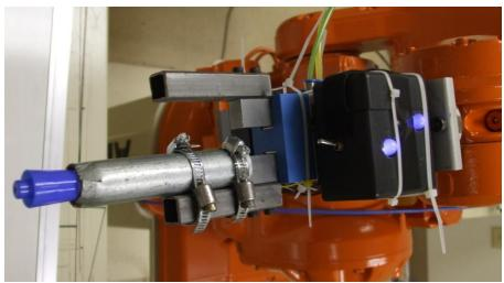
Figure 1: Close up of marker attachment
