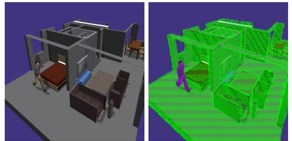
(a) Simulated apartment. (b) Distinction between static and mobile objects.
