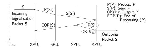
Figure 6: Typical signalling packet processing
