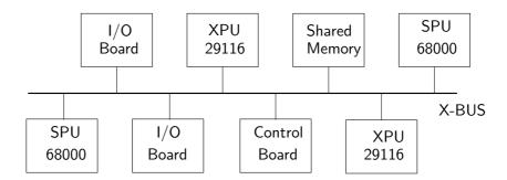
SPU: Signalisation processing unit, XPU: Switching processing unit
