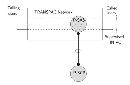
Figure 2: The Intelligent Network Architecture
