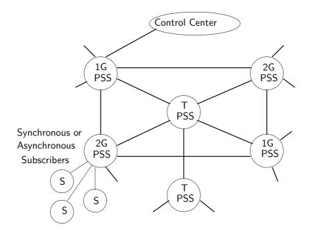
Figure 1: Structure of the TRANSPAC Network
