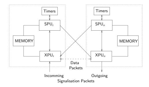
Figure 5: Relations between components during signalling processing
