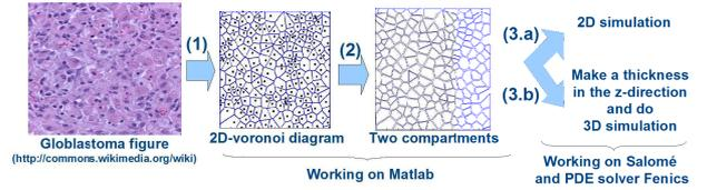
(3.a) Generate the triangular mesh from step 2 using Salomé and perform simulation for 2D using our finite element code.
