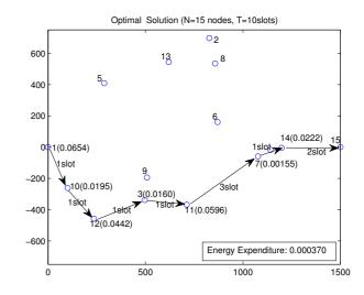
Fig. 3. A sample topology and the result of optimal routing and resource allocation.
