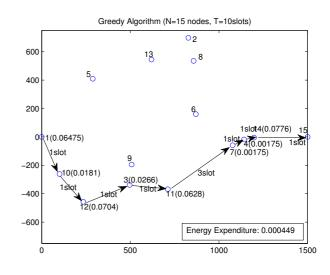
Fig. 4. Result of the greedy algorithm and resource allocation for the same topology
