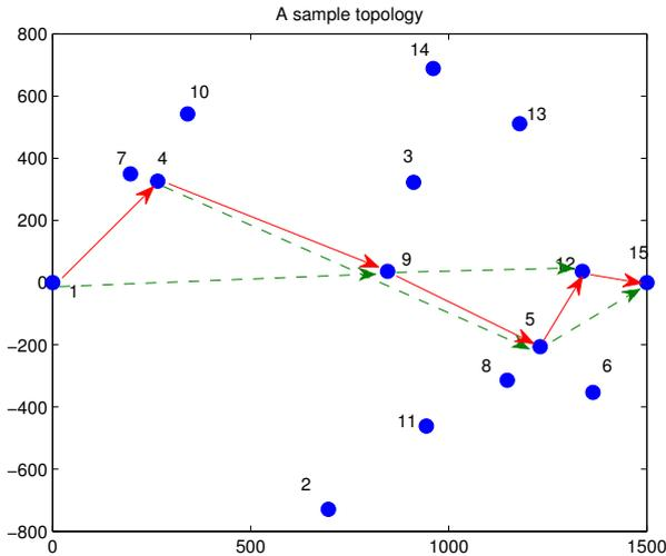
Fig. 1. A sample topology of 15 nodes. Routing path is shown by the solid lines. Each node is also able to accumulate mutual information from the links shown by the dashed lines.
