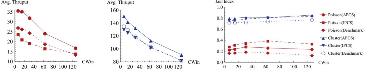
Fig. 9. For independently uniformly random  $\alpha \in [2, 4]$ , the average throughput and Jain index for APCS, IPCS and benchmark under Poisson point model and clustered point model with different contention windows (CWin).
