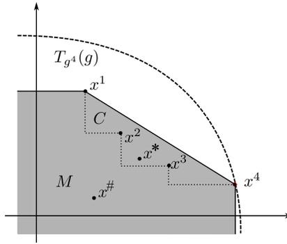
Figure 2. Sets  $C(\mathcal{D}', p)$  (gray area) and  $M(\mathcal{D}', p)$  (subset of gray area left of the dotted lines) for  $p = (-1, -1)$ ,  $\mathcal{D}' = \{(x^i, g^i), i = 1, \dots, 4\}$  and  $g^4 = \mu(\mathcal{D}')$ . The dashed line shows the boundary of the super-level set  $T_{g^4}(g)$ . Point  $x^\#$  represents a test point that allows both m- and c-inconsistency falsification, whereas  $x^*$  allows for c-inconsistency falsification only.
