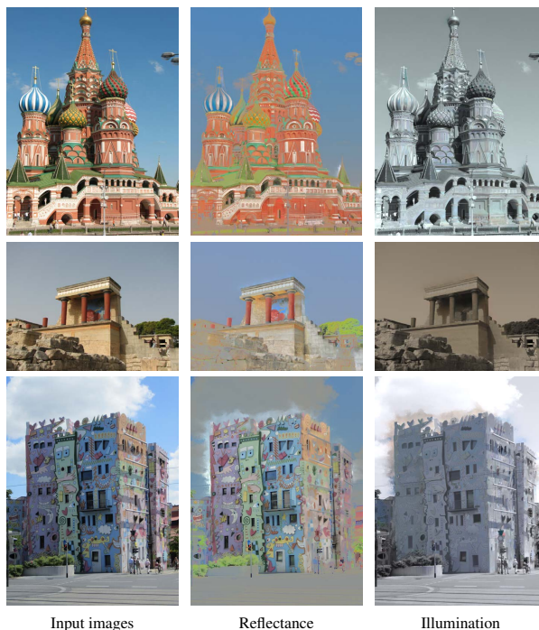
Figure 9: Results of our method on internet photocollections. Top: another view of the StBasil scene. The reflectance we extract is coherent with the one shown in Fig. 8. Bottom: the specular objects which cast shadows on the façade are a challenging case for multi-view stereo. Our method is able to extract their shadows despite the lack of a complete and accurate 3D reconstruction.
