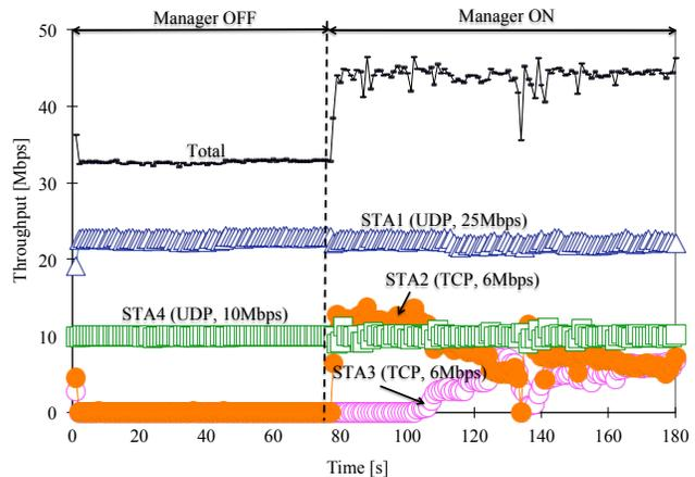
Fig. 16. Throughput of individual STAs for a scenario where STAs with TCP traffic are moved (STA2 and STA3). The TCP traffic could achieve increased throughput at the destination cell.
