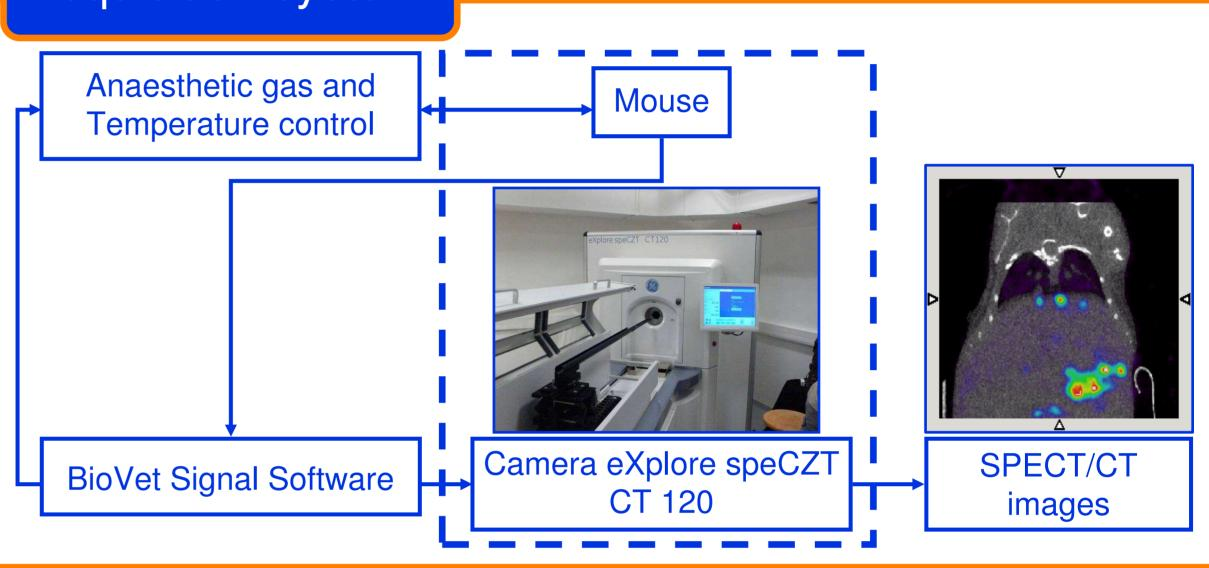
Diagram: The pressure sensor (balloon) is set up under the abdomen of mice. Mice are breathing freely air with anaesthetic gas (Isoflurane). The camera eXplore speCZT CT 120 is a coupling SPECT and CT images. The picture above present liver metastasis from PROb-mNIS adenocarcinoma injected in NOD-SCID mouse.
