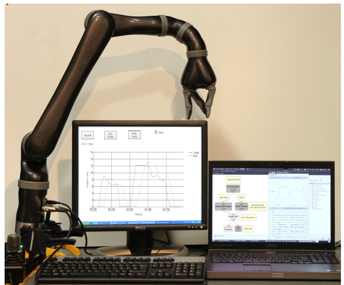
Figure 2: Overview of the experimental setup. OpenViBE (computer on the right side) runs on a linux system to decode intracranial data and send the finger positions to a C# interface (computer on the left side) that translates them into basic commands for the JACO using the API by Kinova. Screen captures of both computers are respectively available as figures 6 and 8.
