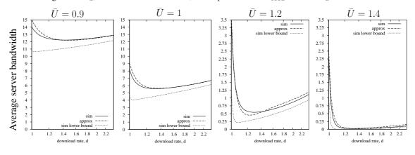
Figure 3: Average server bandwidth as function of the target download rate d, for different values of  $\overline{U}$ , with  $\overline{N} = 100$ ,  $\overline{T} = T_v$ .
