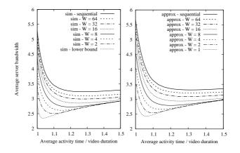
Figure 6: Average server bandwidth as function of the ratio  $\overline{T}/T_v$  between average activity time and video duration, keeping fixed  $\overline{N} = 100$ ,  $d = d_v$ ,  $\gamma = 1$ , for different values of the number of segments W. Comparison between simulation (left plot) and approximate analysis (right plot).
