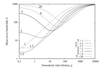
Figure 10: Average server bandwidth Z as function of the normalized video lifetime  $\chi$ , for different values of user activity period  $\overline{T}$ , in the case of  $\Lambda = 1000$ .
