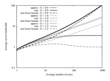
Figure 1: Comparison of average server bandwidth in the case  $d = d_v$ , as function of the average number of users  $\overline{N}$ , for different values of  $\overline{U}$ , in the absence of seeds.
