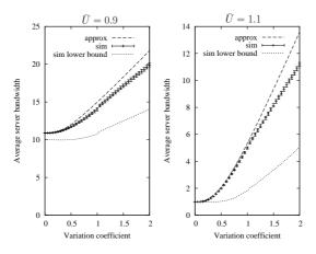
Figure 4: Comparison of average server bandwidth with  $\overline{N} = 100$ ,  $d = d_v$ ,  $\overline{T} = T_v$ , as function of the variation coefficient of peer upload bandwidth, for  $\overline{U} = 0.9$  (left plot) and for  $\overline{U} = 1.1$  (right plot).
