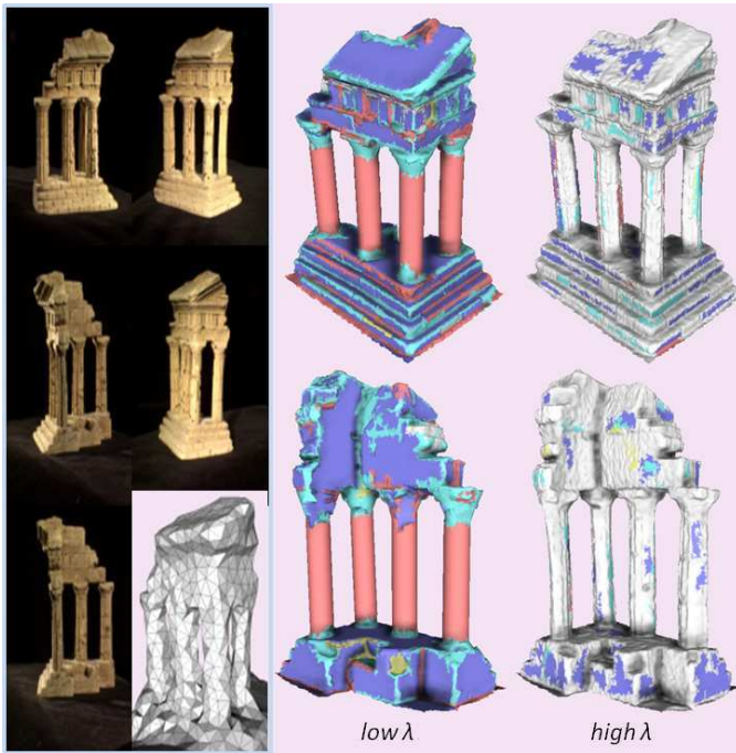
Fig. 12. Impact of the \lambda coefficient from the Temple dataset. Left: input images and a rough visual hull as initial surface; center: result with a low \lambda value; right: result with a high value. Color code: see Fig. 7. The lower the value of the \lambda parameter, the higher the primitives to mesh-patches ratio in the final result. The high \lambda version has a 0.48 mm accuracy and a 99.7% completeness on the Middlebury benchmark [18] whereas the low \lambda version has a 1.03 mm accuracy and a 95.7% completeness. Note that the reconstruction of columns and pieces of walls by cylinders and planes engenders a loss of accuracy in such a case, i.e. when the structures are not regular.
