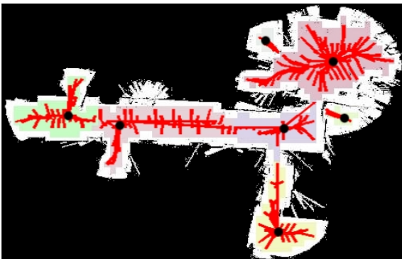
Figure 5: Convergence paths of a subset of grid cells (shown in red) to the corresponding points of locally maximum space clearance (shown in black).
