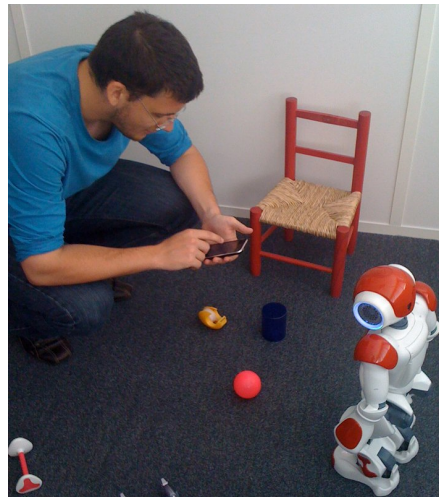
Fig. 1. Using a device as a mediator object between the human and the robot to control the movements of a personal robot allows non-expert users to teach it how to recognize new visually grounded objects.
