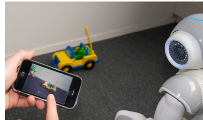
Fig. 4. We display the video stream of the camera of the robot on the screen. This allows accurate monitoring of what the robot is seeing.
