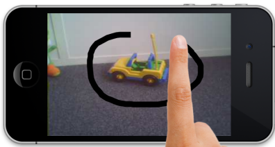
Fig. 6. Once the user asks the robot to take a picture of a new object, he can directly encircle it and thus providing a useful rough object segmentation.
