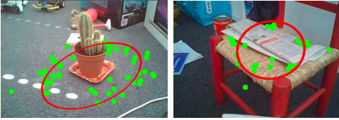
Fig. 10. Encircling with a laser pointer raises difficulties mostly due to the projection of the laser spot in the plane of the camera.
