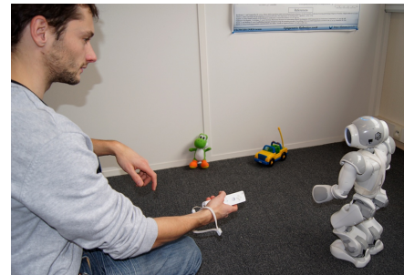
Fig. 7. Users can move the robot by using the directional cross or directly orienting the Wiimote to aim its head. However, the lack of feedback makes it very difficult to estimate whether the robot really sees the object the user wants to teach.
