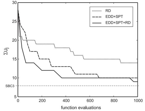
**Fig. 6:** Exemplary best results for  $P_8|d_j|\sum U_j$  and several operator combinations and the result of the SBC3 heuristic ( $\sum U_j = 8$ ). First, only a random mutation operator is applied to the population (RD). Second, EDD and SPT inspired operators are applied (EDD+SPT). Finally, all operators are combined (EDD+SPT+RD).
