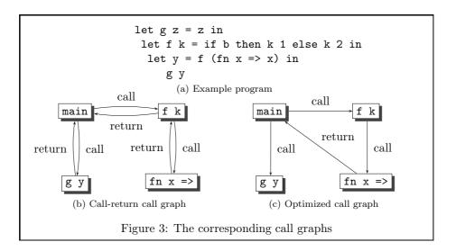
style CFA gives rise to Figure 3b, where we have named the main expression of the program main. In addition to the above resolved call, our analysis will determine that the anonymous function returns to the let-binding of y in main upon completion, rather than to its caller. The analysis hence gives rise to the more precise control-flow graph in Figure 3c.
