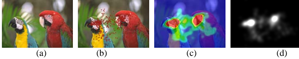
Figure 3: From left to right, (a) Original (b) Fixation map with red fixation points (c) Heat map (red spots represent the most visually salient areas of the picture) and (d) Saliency map.
