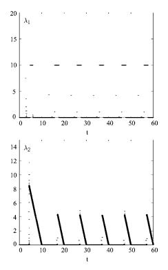
Fig. 8. Up: Variation of the contact force during the motion on  $\Sigma_1$ ; Down: Variation of the contact force during the motion on  $\Sigma_2$ .
