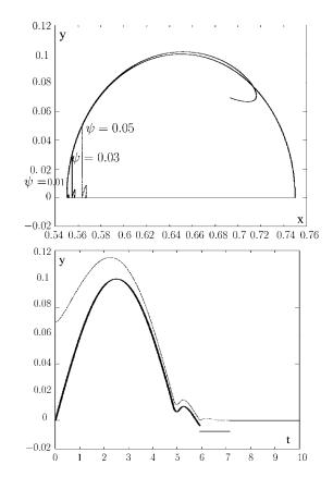
Fig. 4. Up: The influence of  $\psi$  on the real trajectory's deformation for controller's gains set to  $\gamma_1 = 8$ ,  $\gamma_2 = 7$ . Down:  $y(t) = q^1(t)$  (dashed) and  $y_a^*(t) = (q_a^1)^*(t)$  (solid) during the first cycle ( $\psi = 0.01$ ).
