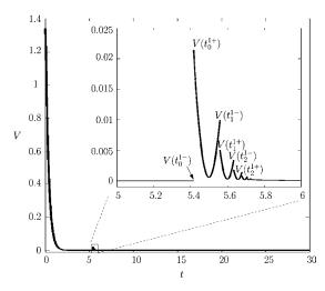
Fig. 6. Variation of the Lyapunov function for  $\gamma_1 = 8$ ,  $\gamma_2 = 7$ ; Zoom: Variation of the Lyapunov function during the phase  $I_0$ .
