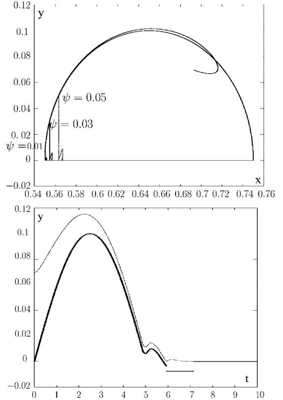
Fig. 4. Up: The influence of  $\psi$  on the real trajectory's deformation for controller's gains set to  $\gamma_1 = 8, \gamma_2 = 7$ . Down:  $y(t) = q^1(t)$  (dashed) and  $y_d^*(t) = (q_d^1)^*(t)$  (solid) during the first cycle ( $\psi = 0.01$ ).
