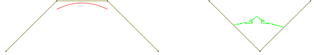
Figure 9. Left: cubic spline with 4 control points. Right: a fractal curve with 3 control points.
