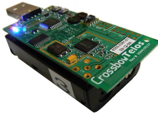
Figure 10: The TelosB mote.
