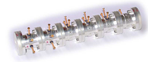
Fig. 1. A microwave filter.
