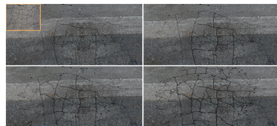
Figure 10: From left to right and top to bottom: Road model showing fracture propagation, simulating the course of time.
