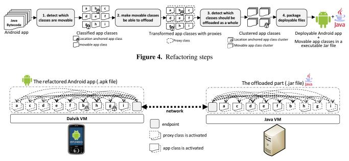
Figure 5. The runtime architecture of an offloaded Android app
