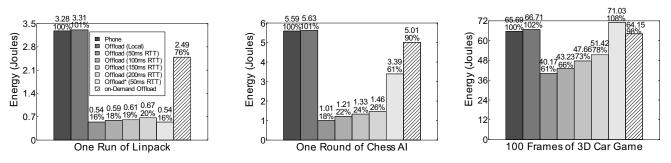
Figure 12. The power consumption comparison of the Android apps running in different scenarios
