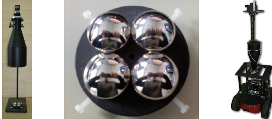
Figure 1: The omnidirectional stereo sensor we used: orthographic camera, parabolic mirrors, 90 cm height
