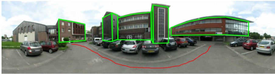
(a) environment; red: an idea of the robot path; green: tracked edges in (d-f)
