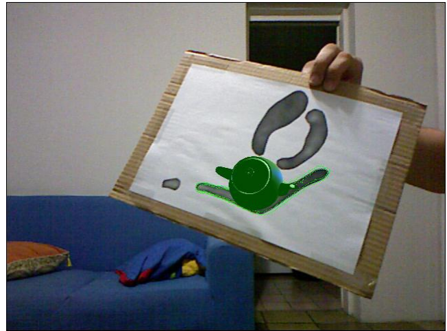
Figure 1: Augmentation of the ISMAR logo using the DARC method. The highlighted contour is rectified with the aid of depth data, allowing its detection and pose estimation.
