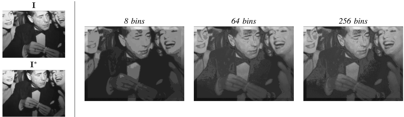
Fig. 3. Influence of the number of bins on the predicted image when far from reach. On the left, with 8 bins the image is flattened and has lost a lot of high frequencies. 256 bins introduces more noise when the difference between \mathbf{I} and \mathbf{I}^* increases than 64. The frame on the borders represent the area in the image which is not included in the computation.
