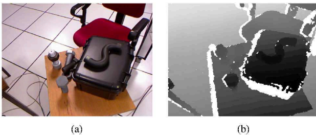
Fig. 2. Example of static scene (a) and corresponding depth map representation (b) acquired from Microsoft Kinect sensor. The darkest pixels correspond to the smallest depths. White pixels correspond to unavailable data.
