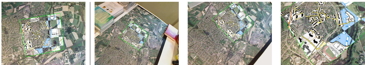
Fig. 11. Registration of an aerial sequence with a map template image by MI: frames 1, 250, 500 and 750 are represented with the over-imposed satellite reference (inside the green rectangle) projected using the estimated homography (image and map source: IGN) .
