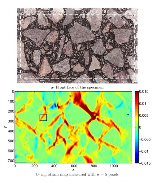
Figure 14: Asphalt specimen under compression [15]
