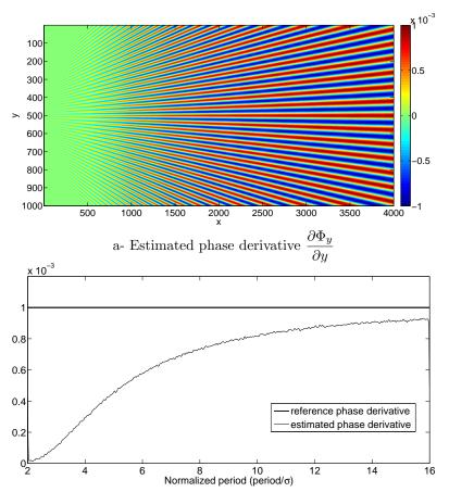
b- Cross-section of the estimated phase derivative map along the x-axis
