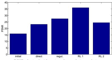
a- PSNR obtained with various deconvolution techniques
