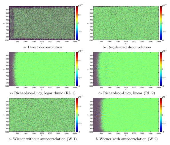
Figure 7: Difference between deconvolved and reference phase derivatives obtained with various deconvolution strategies. Noise amplitude=3
