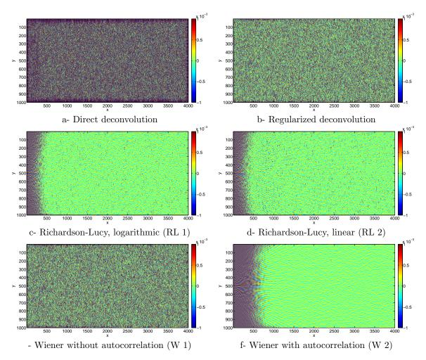
Figure 8: Difference between deconvolved and reference phase derivatives obtained with various deconvolution strategies. Noise amplitude=5
