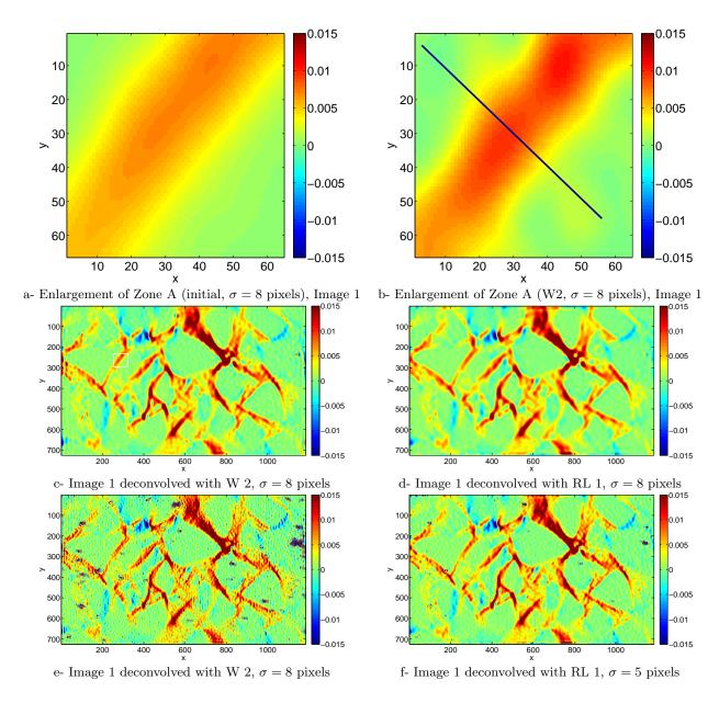
Figure 15: Asphalt specimen under compression. Deconvolution of Image 1 for load level 1
