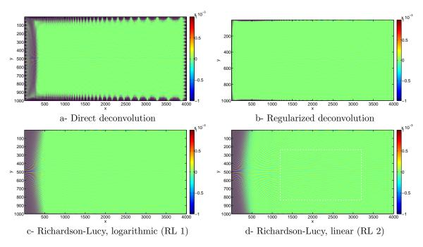
Figure 5: Difference between deconvolved and reference phase derivatives obtained with various deconvolution strategies. Noise amplitude=0
