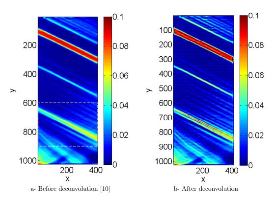
Figure 18: Shape memory alloy under tension.  $E_{yy}$  map  $\left[10\right]$
