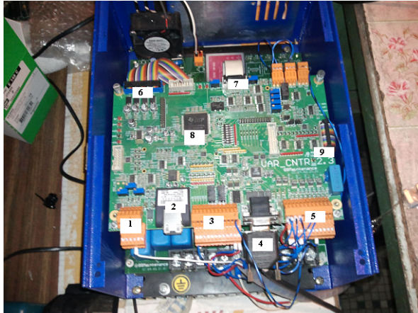
Fig. 6. VAR-CNTRL card a product of GS Maintenance.
