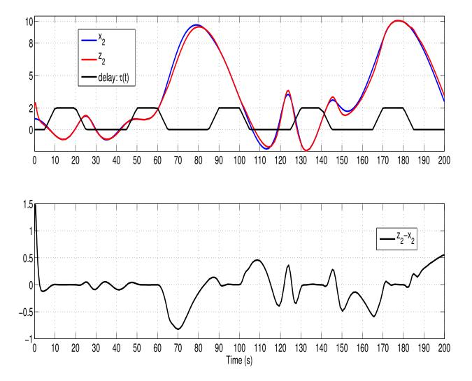
Fig. 1.  $x_2$  and its estimate  $z_2$ , time-varying delay  $\tau(t)$  and observation error  $(z_2 - x_2)$ .
