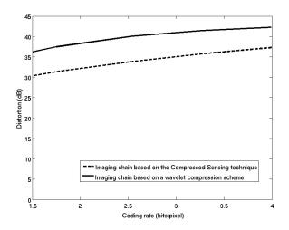
**Fig. 3**. Rate-distortion function for the two acquisition techniques. The dashed curve is the PSNR w.r.t. the compression rate for the CS acquisition technique while the solid curve is the PSNR w.r.t. the compression rate for the wavelet-based method.
