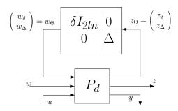
Fig. 2. LFR system depending on system parameters and sampling period variation
