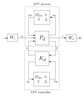
Fig. 3. LFR control structure
