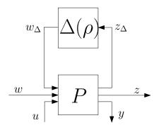
Fig. 1. System under LFR form
