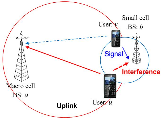
Figure 2: The signal received at BS  $b$  sent from user  $v$  can be strongly interfered by the transmission of user  $u$  since  $u$  has to use a relatively high power in order to send its signal to BS  $a$  in long distance.
