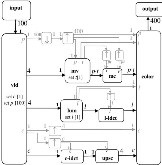
Fig. 6. Video decoder (compiler-inserted elements shown in gray).
